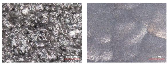
(a) Without treatment (b) With treatment Fig. 1 Aspect of surface of titanium alloy manufactured by electron beam melting EBM
