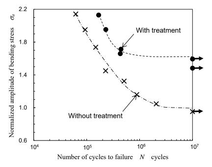
Fig. 2 Improvement of fatigue strength of titanium alloy manufactured by EBM
