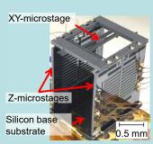
Assembled 3D scanner for LT measurement
