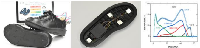
Gait analysis using sole sensor system (Photo by Denjiken)
