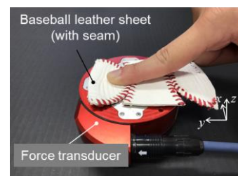
Evaluation of frictional properties of friction aids for sports
