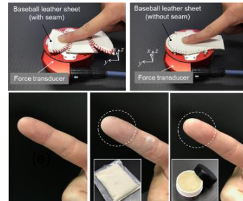
Evaluation of frictional properties of friction aids for sports
