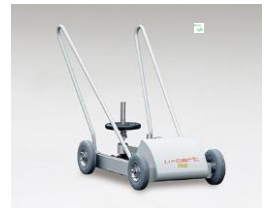
Slip-resistance testing device
