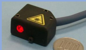
Laser angle sensor for extremely small angle ( 1/10000^\circ )
