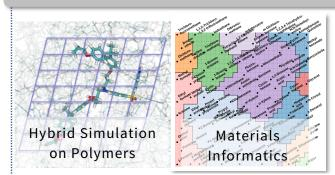
As for development of polymeric materials, designing various properties by controlling the molecular-scale structure and phase separation is being required. Using integrated numerical analyses covering molecular-scale to macroscale phenomena and machine learning-aided informatics techniques, we aim to explore and design polymeric materials.
