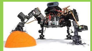
Rock-Climbing Robot for Lunar Skylight Exploration
