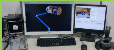
Dynamic Simulator for HTV Capture by Space Manipulator
