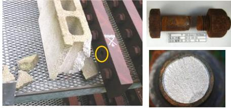
Fracture of an exposed high strength bolt caused by hydrogen entry due to corrosion
