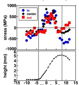
Residual stress distribution in a stretch-formed specimen
