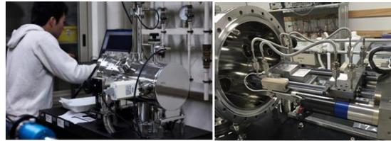
An apparatus to detect hydrogen during tensile test
