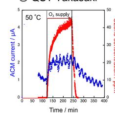
Acceleration of corrosion by ozone
