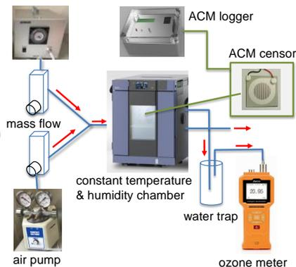
Corrosion monitoring using an ACM sensor in a corrosion test chamber with introduced ozone
