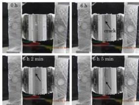
Evaluation of HE property of high strength steel sheet simulating press forming
