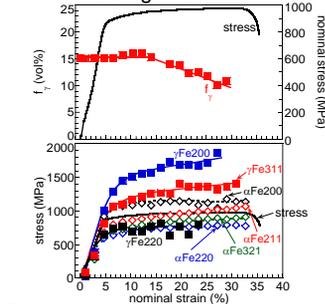
Transformation behavior in the residual  $\gamma$  (upper) and stress partitioning behavior in  $\alpha$  and  $\gamma$  phases (lower)
