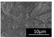
Surface of ceramic coating for use in supercritical water environment.
