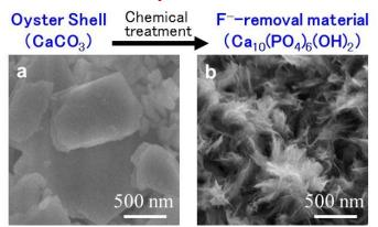
Preparation of  $F^{-}$ -removal material from oyster shell. Oyster shell (a) before treatment and (b) after treatment.
