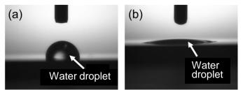
Water droplets on the substrate surface coated with photocatalytic ceramics. (a) before UV irradiation, (b) after UV irradiation.
