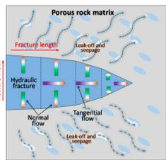
CO<sub>2</sub> & water fracturing is still effective with the pre-existing pore water and is particularly effective in porous volcanic rocks.
