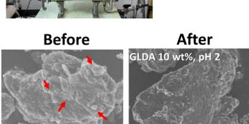
Montmorillonite dissolved in GLDA Confirmation of pore formation
