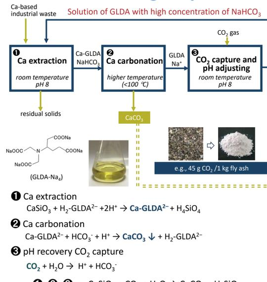
CCUS [Carbon dioxide Capture, Utilization and Storage] → CO<sub>2</sub> mineralization
