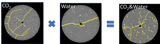
CO<sub>2</sub> & water fracturing mechanism
