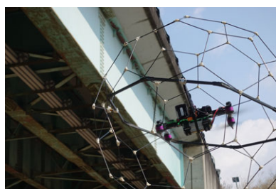
Passive rotating spherical shell drone for infrastructure inspection
