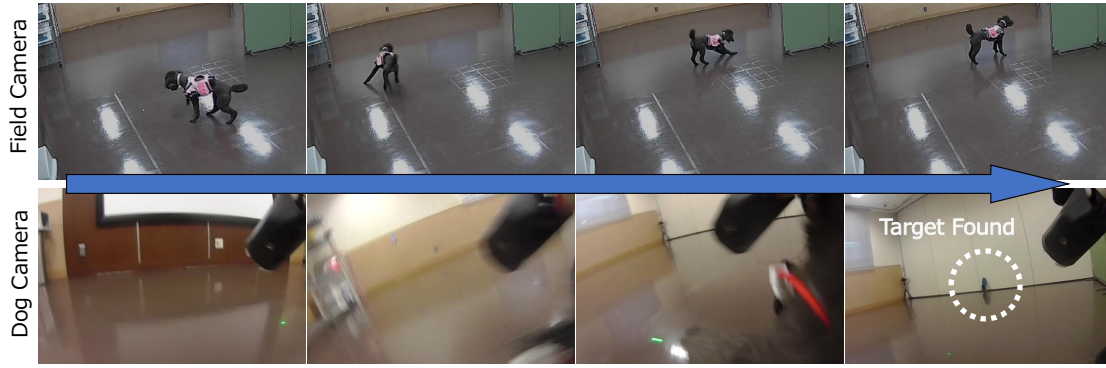
Fig. 14. Navigation of a canine by using 3 laser beams: Upper figures show the canine's motion. Lower figures show the on-suit camera images. Operator controlled the canine's moving direction by a joy-pad. Canine moved beyond partition panel and took images of target object.
